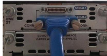
Imagen 6.60 “Cable serial DTE R2”
