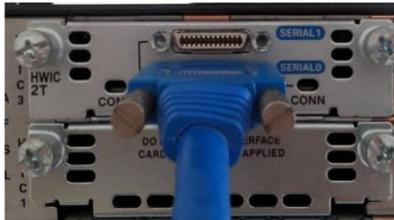
Imagen 6.59 “Cable serial DCE R1”
